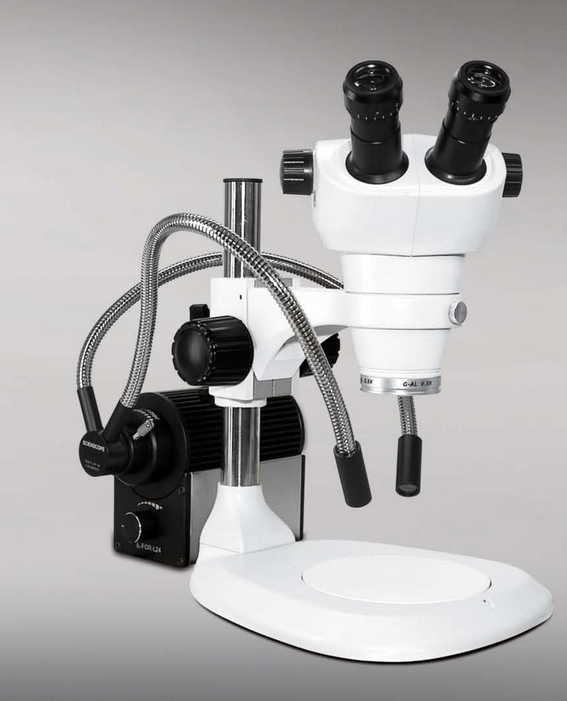
Package Contents NZ binocular body 0.5X objective lens Post stand 10X eyepieces
